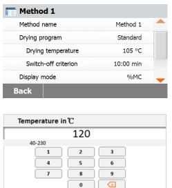
Press the **Drying Temperature** button to access the temperature setting menu.
