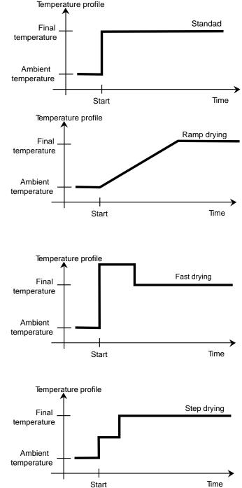
An alternate application possibility lies in the selective determination of the moisture at different temperatures. Gypsum, for example, releases only its surface water at 50°C,
