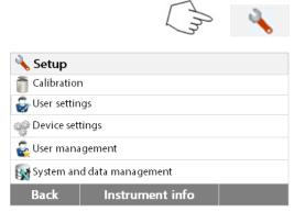
Press the **Setup** button to access the Setup menu. Press **Back** to return to Home screen.
