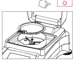
If the display is not visible and the unit is plugged into a power source, press the On/Off button.
