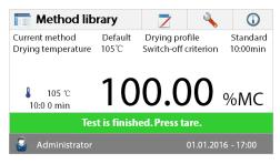
The display indicates the Method Name, Temperature/Time, actual temperature, elapsed time duration of the test, moisture and curve. The test automatically stops at the end of the measurement. If you want to end the test sooner, press the button.
