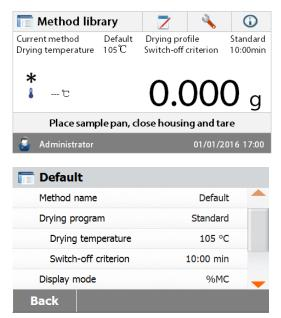
The analyzer comes with a default method preinstalled. Follow the instruction message to start a measurement directly. Press parameters area to edit.
