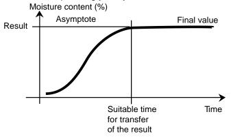
In the second type, drying runs quickly at the start and then flattens out. The moisture content never assumes a constant value. The causes of such a drying profile can be as follows:
