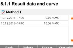
Press result item to access the detail data. Press **Back** to return to previous step. Press **Delete** to delete the results. Press **Export** to export these results. Press Statistics to access statistics menu.
