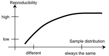
The final results of a moisture determination depends on a carefully thought out sample preparation. The part of the sample used for analysis must always be representative of the total quantity. The sample preparation includes work processes such as sampling, sample division, size reduction, homogenization and others. All of these processes should be carried out as quickly as possible and without loss or uptake of moisture.
