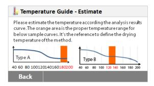
The analysis will finish with a characteristic curve calibrated by a temperature axis. Press **Temperature Estimate** button to compare the result curve with typical curve guide.
